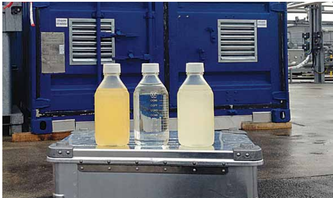
Water samples taken during a long-term run on a gas field site, from left to right: raw produced water, effluent after treatment, pre-treated water
